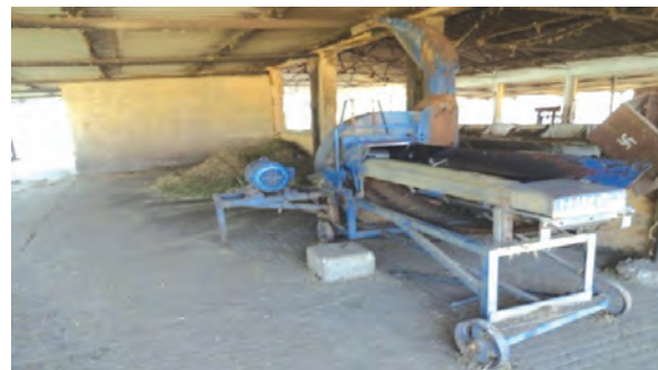
(e) Different type of electrically operated chaff cutter
