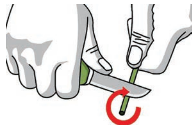
Fig. 9.27 Roll the wire with one hand
