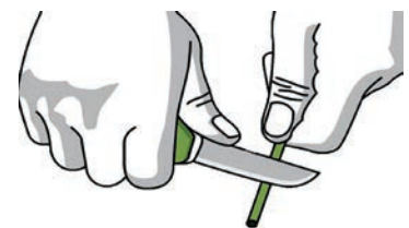
Fig. 9.26 Place a utility knife on the wire that needs to be cut
