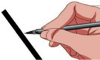
Fig. 9.29 Marking on the wire for bending
