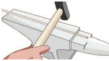
Fig. 9.42 Straightening the wire using a hammer
