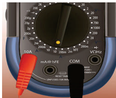
Fig. 7.9 Probes of multimeter connected to current measurement slot
