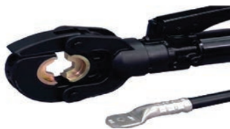
Fig. 9.72 Crimped cable with crimper
