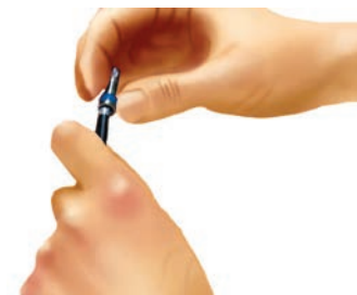
Fig. 9.15 Insert a connector in the cable conductor
