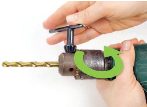
Fig. 7.21 Turn the chuck key counter clockwise
