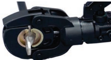
Fig. 9.70 Inserting the cable into the crimper
