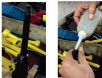
Fig. 9.60 Fill oil in the hydraulic crimping tool
