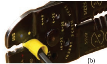
Fig. 9.64 (a and b) Squeeze the handle of the crimper to crimp the connector
