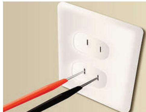
Fig. 7.6 AC voltage measurement
