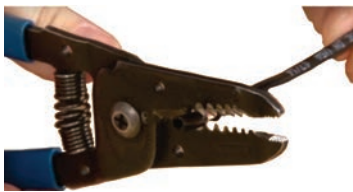
Fig. 9.61 Strip off the insulation
