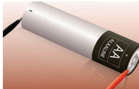
Fig. 7.7 DC Voltage measurement
