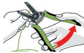
Fig. 9.21 Press the handles of the stripper to remove insulation
