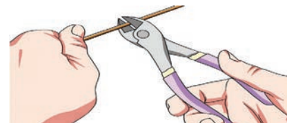
Fig. 9.50 Cutting the extra wire with a wire cutter
