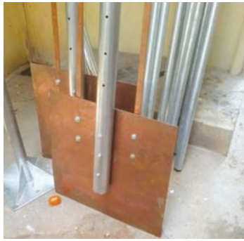
Fig. 4.8 Copper plate used for plate earthing
