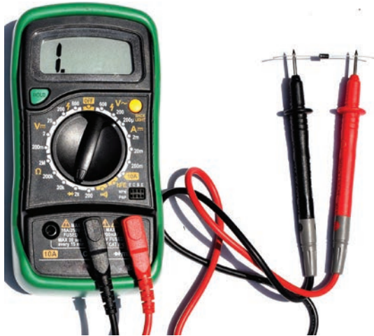
Fig. 2.32 Diode in reverse bias condition
