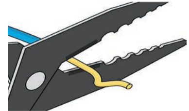
Fig. 9.25 Cut the damaged part of the wire
