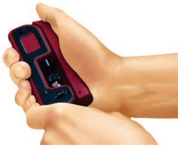
Fig. 9.16 Crimp the connector using a cable crimper
